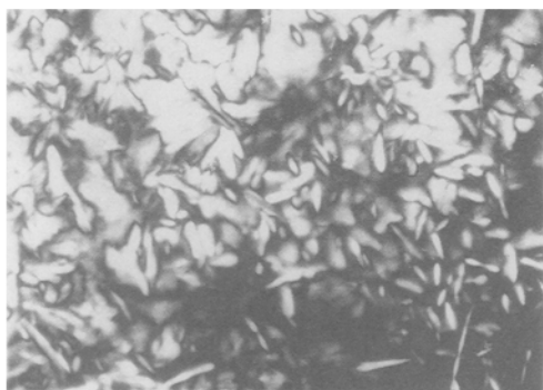
FIG. 3. Liquid crystalline structures formed in the water/ N^{\alpha}N^{\alpha'} bis(N-lauryl N,N dimethyl glycine) cystine dimethyl ester dihydrochloride system: a, hexagonal structure; b, crystalline phase.
