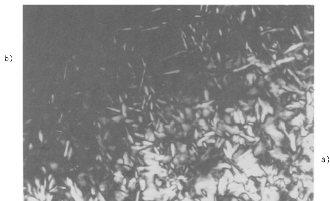
FIG. 3. Liquid crystalline structures formed in the water/ N^{\alpha}N^{\alpha'} bis(N-lauryl N,N dimethyl glycine) cystine dimethyl ester dihydrochloride system: a, hexagonal structure; b, crystalline phase.
